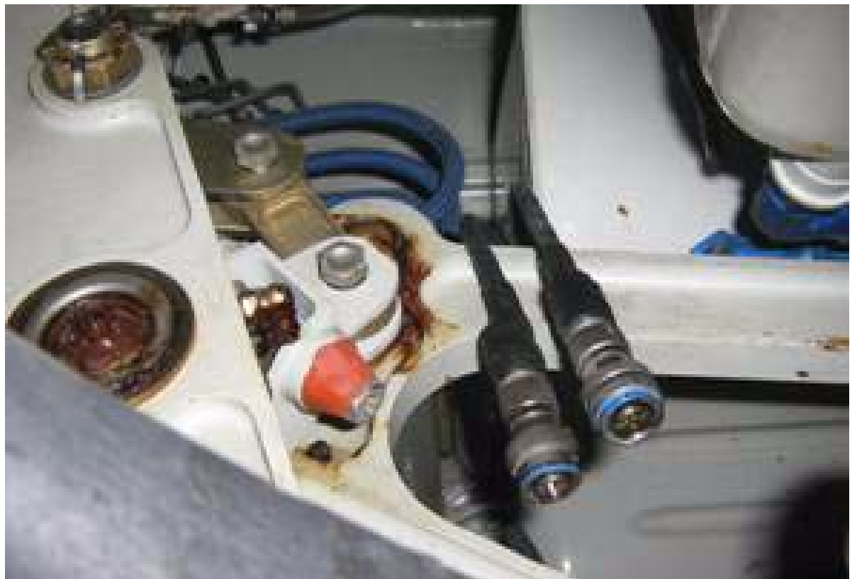
Fig. 507 - Main Landing Gear Limit Switches - Electrical Test and Cleaning (Sheet 2 of 5)
