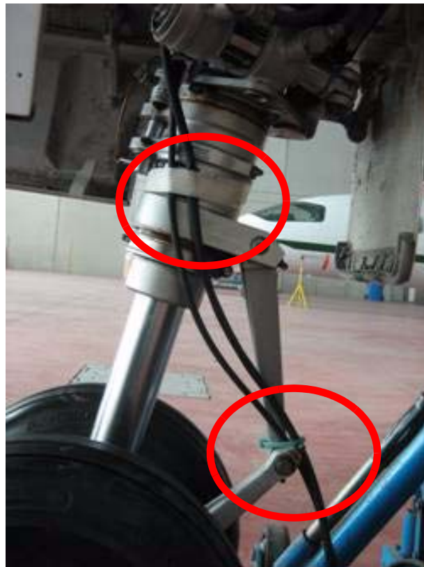
Fig. 507 - Nose Landing Gear Limit Switches - Electrical Test and Cleaning (Sheet 4 of 5)
